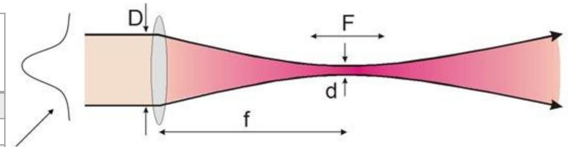
$$I(r) = I_0 \exp(-2r^2/w^2) = I_0 \exp(-8r^2/D^2) \quad \text{Numerical aperture } NA = \sin(D/2f)$$
