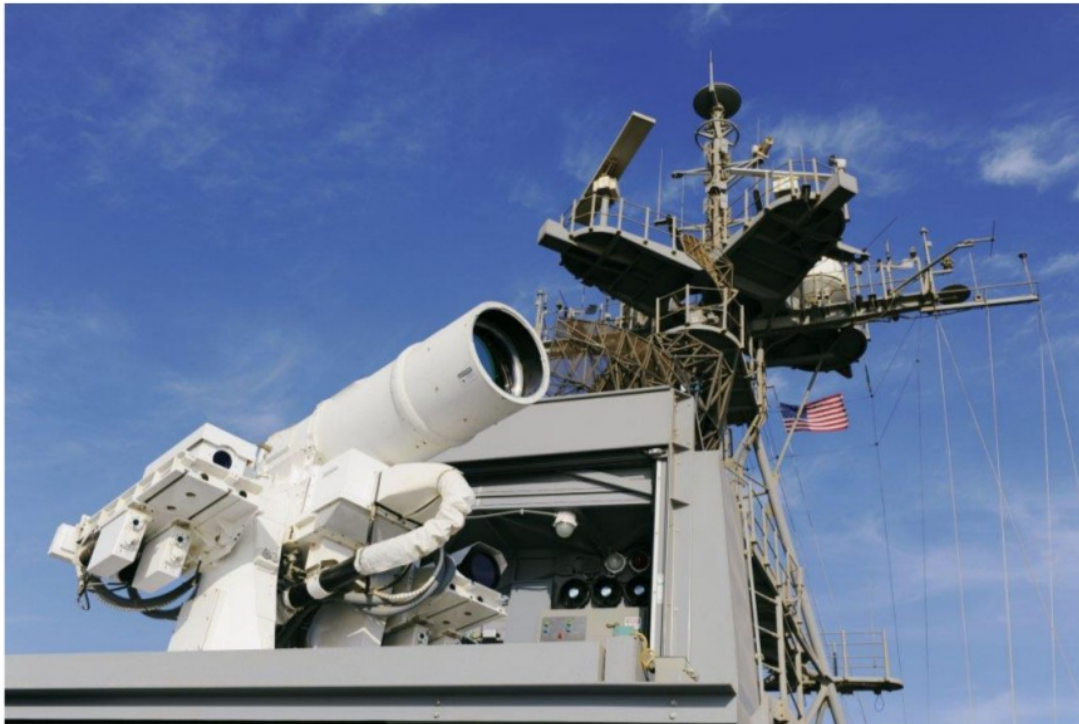
The 33 kW beam-superimposing fibre-based solid state LaWS was tested in the Gulf on board USS Ponce in 2014. (US Navy)
